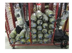
Scott Carbon Wrapped 4500 psi Cylinder Air Tanks
